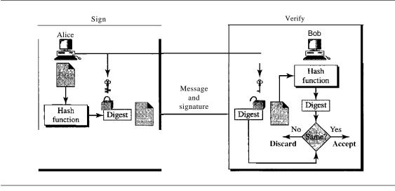
Figure 31.12 Signing the digest in a digital signature
