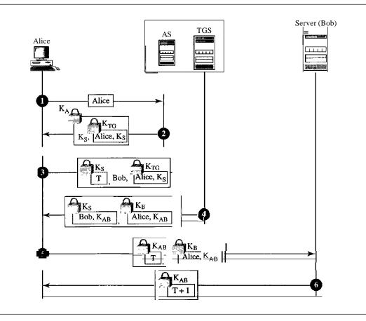
not stay in the terminal. It is only used for a moment to create  $K_A$ . The process now uses  $K_A$  to decrypt the message sent. Both  $K_S$  and the ticket are extracted.
