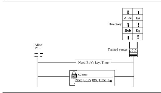
Figure 31.25 Controlled trusted center
