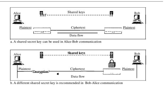
Figure 31.2 Message confidentiality using symmetric keys in two directions
